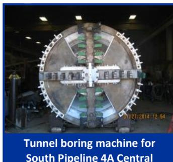
Tunnel boring machine for South Pipeline 4A Central
